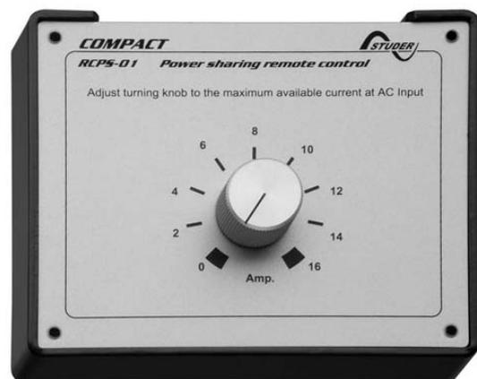
**Caution: the COMPACT will not limit if an appliance draws more current than available from the source ! This means that the connected generator will be over-loaded or that the circuit-breaker before the COMPACT will break.**
