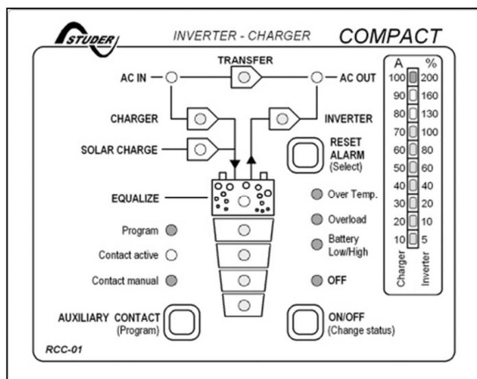
The output power and the charging currents are displayed on the Remote Control. In the Remote Control there is an additional Alarm Contact and a built-in Control Input. These two functions are available through Tip-jack RJ11/4 for use. This Auxiliary Contact is Front / Work Contact (max. 0.5A!), which is independent from the Auxiliary Contact of the COMPACT. This contact is active in case of an alarm of the COMPACT.
